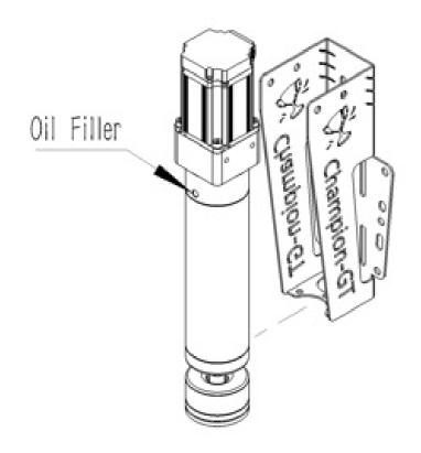
Align the two M6 threaded holes on each side of the Actuator with the holes in either side of the U-Shaped Bracket.
